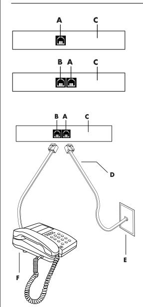
To connect the cable between the modem and the telephone service line:
